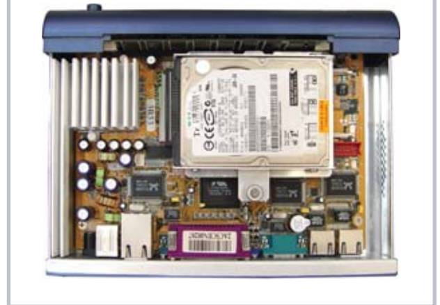
LIGHT Chassis without top-cover
